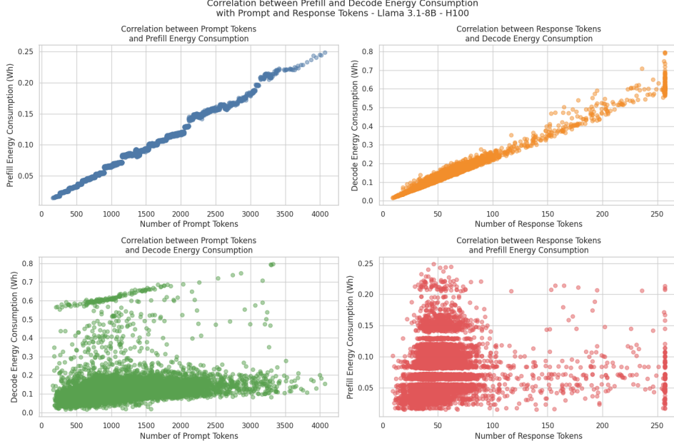
Figure 5: Correlation between token lengths and GPU energy consumption in prefill and decode phases.
